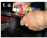
d. The fit is very snug. If it is difficult to push the finger into the receptor, spray receptor piece of the finger with a multi-purpose lubricant (such as WD-40).
