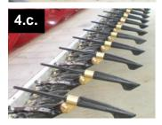
c. Set all the lifters to be the same angle; they should form a straight line when you look down the row. It is important that all lifters are working in unison. Retighten the receptor lock nut and carriage bolt on all lifters.
