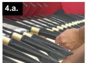
a. Loosen the receptor's lock nut from the carriage bolt and adjust the angle of the nylon finger.
