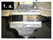
a. Place the lifter in a vise with the rail spring pointing towards the ceiling.
